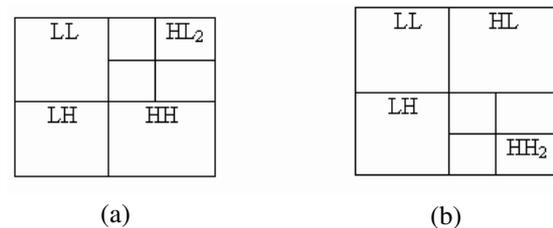
Fig. 1.4: Multi-resolution DWT sub-bands of the original image
