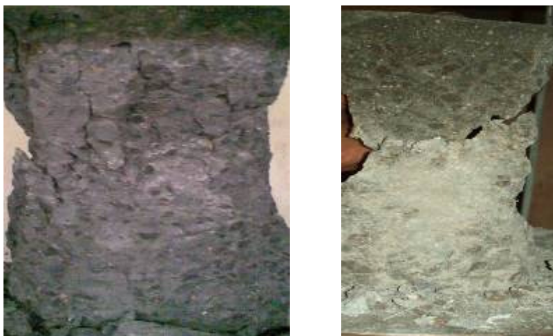
Fig. 7.5. Ultimate Cracking pattern of cylinders
