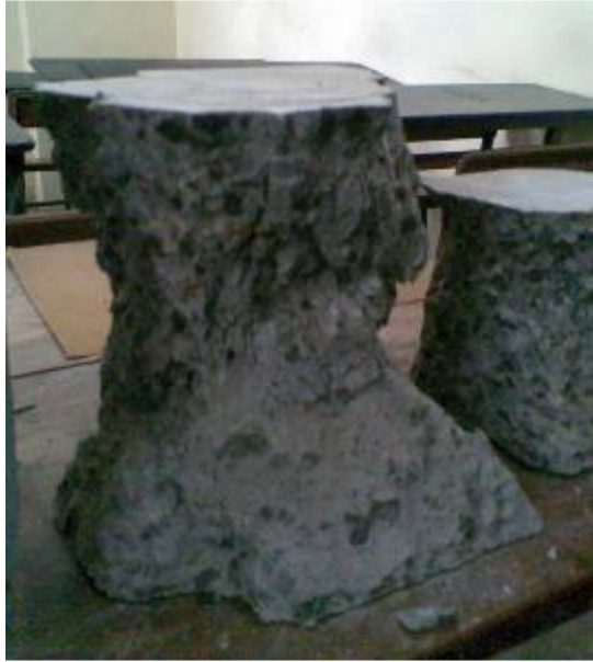
Fig. 7.3 Ultimate Cracking pattern of Cubes
