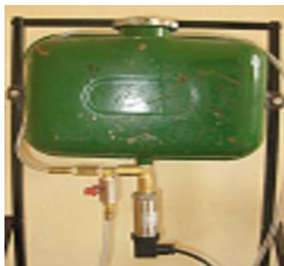
Fig.3 Fuel Tank Unit
