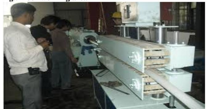
**Fig.6 Improper arrangement of supporting tools**
