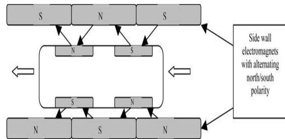
Fig.1. Magnetic Levitation
