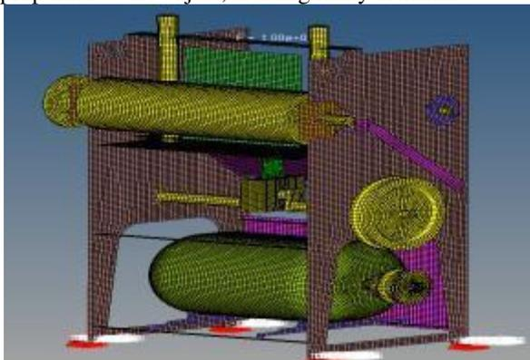
Fig. 6. Finite Elemental Analysis Model
