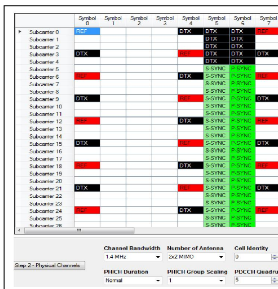
Figure-6.6 Physical channel 2x2 MIMO
